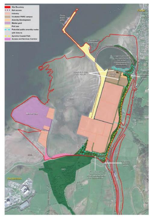
7.7.5 The above diagram, taken from the Hunterston PARC Framework, shows the proposed development framework with the layout of uses for the site, including Industry, Port use and transport links.
